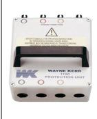
High precision component measuring instruments can be destroyed by charged capacitors - leading to expensive repairs and unacceptable downtime. The 1100 Protection Unit is designed for use with the 6430B or 6440B Component Analyzers to provide protection up to 25 Joules. In the event of an overload a fuse blows and the test equipment remains unharmed.
