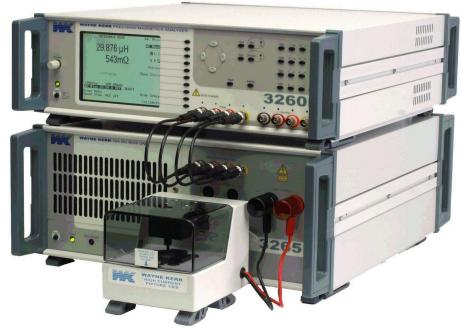
SMD inductors can be tested with DC bias currents up to 50A by using the High Current Fixture accessory with the 3260B Precision Magnetics Analyzer with either one or two 3265B DC Bias Units
