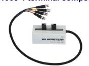
Remote test fixture for axial, radial or bandoliered components. Complete with cable terminating in four BNC connectors.
