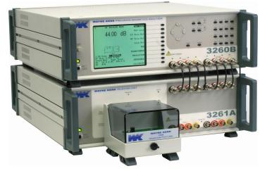
3261A Telecom Unit is the core of a comprehensive test system which incorporates 3260B Precision Magnetics Analyzer and is enhanced by Telecom Fixture model 1008
